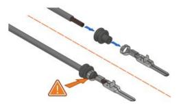
4. Noting the polarity, insert the crimped spade terminals into male connector (removed in step 1) as shown. Ensure the cables are fully located - retaining catches will click into place.
