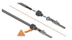
4. Noting the polarity, insert the crimped spade terminals into male connector (removed in step 1) as shown. Ensure the cables are fully located - retaining catches will click into
