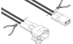
2. Remove ¼" (6mm) of cable shroud to reveal the wire core. Crimp the female spade connectors as shown.
