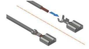
3. Noting the polarity, insert the crimped spade terminals into the supplied RTB-2 connector as shown. Ensure the cables are fully located - retaining catches will click into place.
