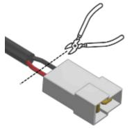
Slide the cables through the supplied rubber seals before removing ¼" (6mm) of shroud to reveal the wire core. Crimp the male spade connectors, noting the rubber seal position, as shown.
